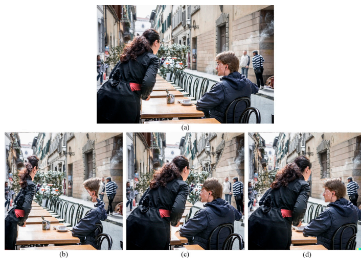
Figure 7. Original image (a), retargeted image using naïve seam carving (b), our proposed hybrid energy method (c), and retargeting the subjects separately from the rest of the image using the proposed layered method (d). The layered method uses SAM and CLIPSeg to segment the layers, and DALL-E is used to inpaint the missing areas of overlap. The layered method results in significantly less distortion to the background, and better preserves the primary subjects in the image.
